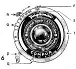
Compur (fig. 6), Prontor II (fig. 7), Pronto (figs.8 and 9) must be set by pressing the lever *n* in the direction of the arrows. Do this for all adjust-
