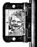
more the exact size of the actual picture. As figure 22 shows, the actual picture will be displaced towards the camera-edge by 1/6 (distance between camera and object not under 20") or by 1/4 (distance between camera and
